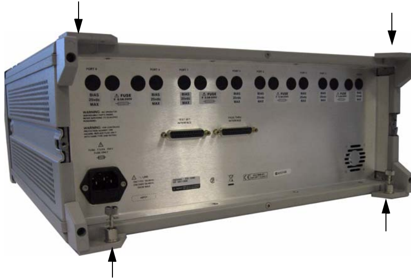
Figure 14 Installing Lock Feet
